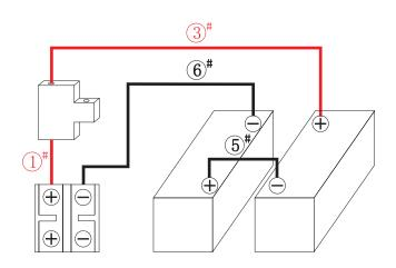
Note: Don't reverse battery polarities, or battery will be damaged
