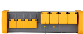
VFL launching port
